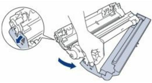
6. Reinsert the toner cartridge firmly into the new drum unit until you hear it lock into place.
