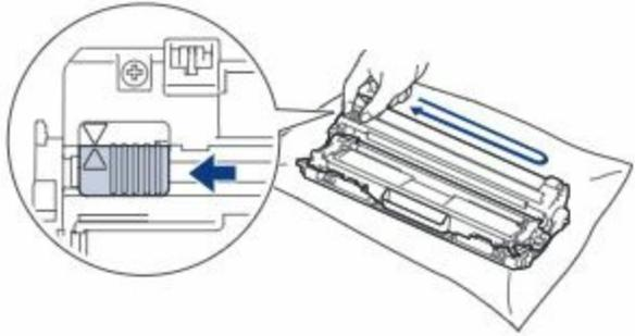
*Be sure to return the green tab to the Home position (▲). The arrow on the tab must be aligned with the arrow on the drum unit. If it's not, printed pages may have a vertical stripe.*
