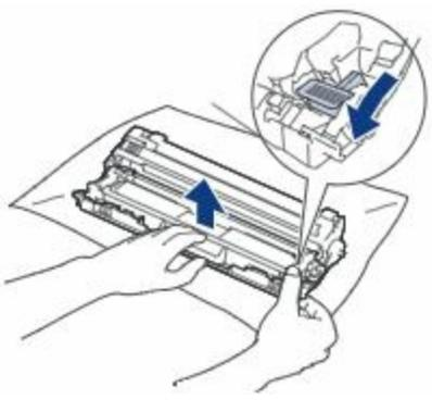
5. Unpack the new drum unit and remove the protective cover.
