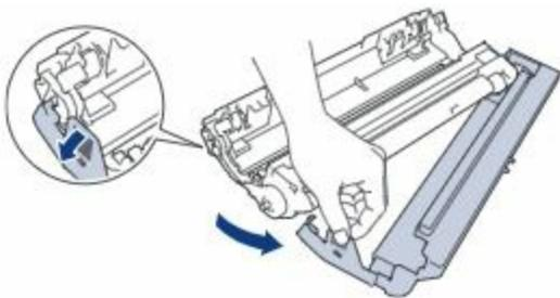
6. Reinsert the toner cartridge firmly into the new drum unit until you hear it lock into place.
